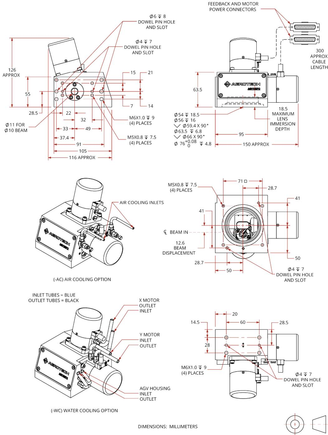
**Figure 2-5: AGV14XPO-E1-BE1 Galvanometer Scanner Dimensions**
