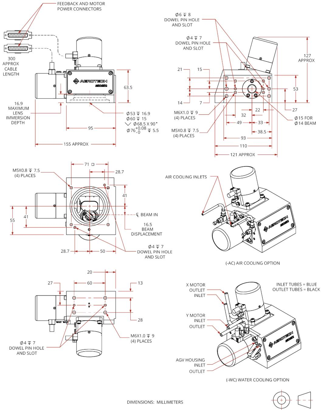
Figure 2-6: AGV14XPO-E1-BE2 Galvanometer Scanner Dimensions
