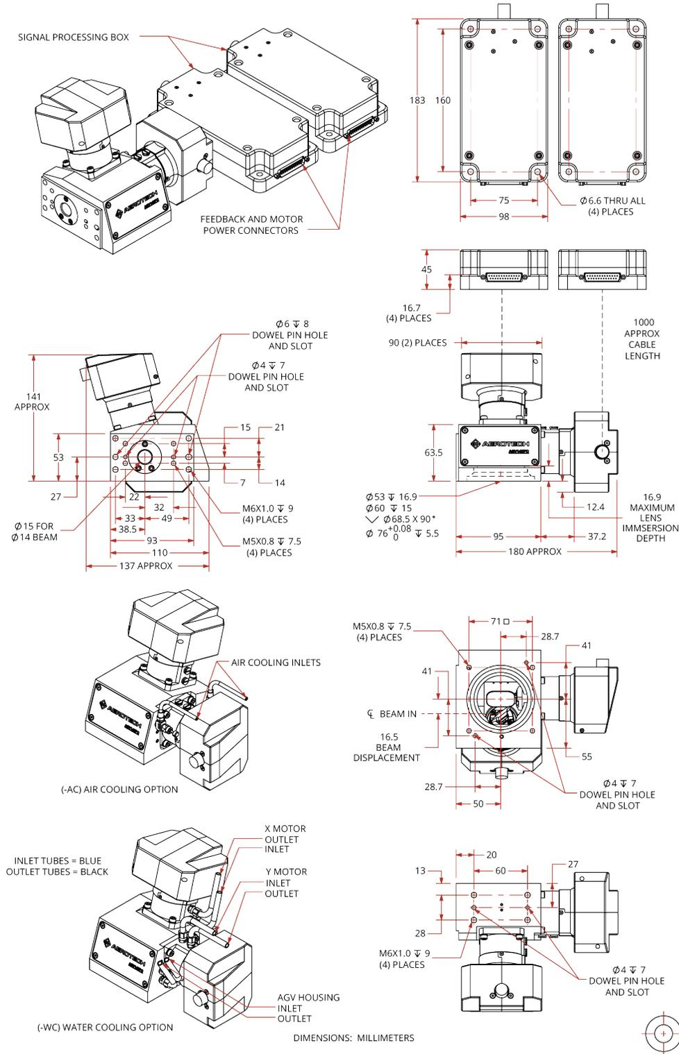
**Figure 2-9: AGV20XPO-E1-BE1 Galvanometer Scanner Dimensions**
