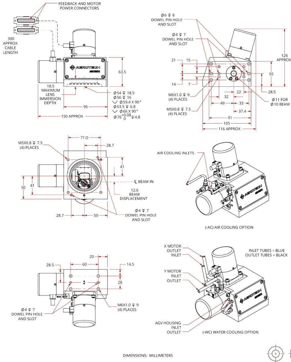
Figure 2-2: AGV10XPO-E1-BE2 Galvanometer Scanner Dimensions
