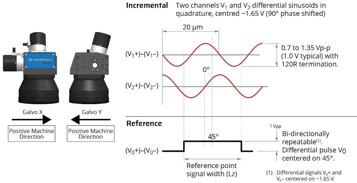
Figure 3-5: -E2 Option Encoder Phasing Reference Diagram
