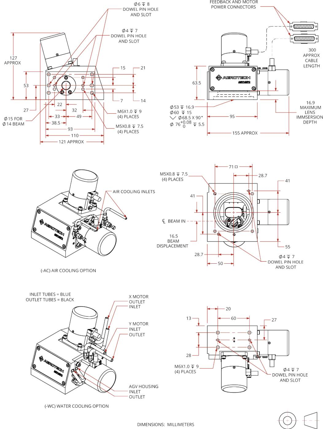
Figure 2-7: AGV14XPO-E2-BE1 Galvanometer Scanner Dimensions
