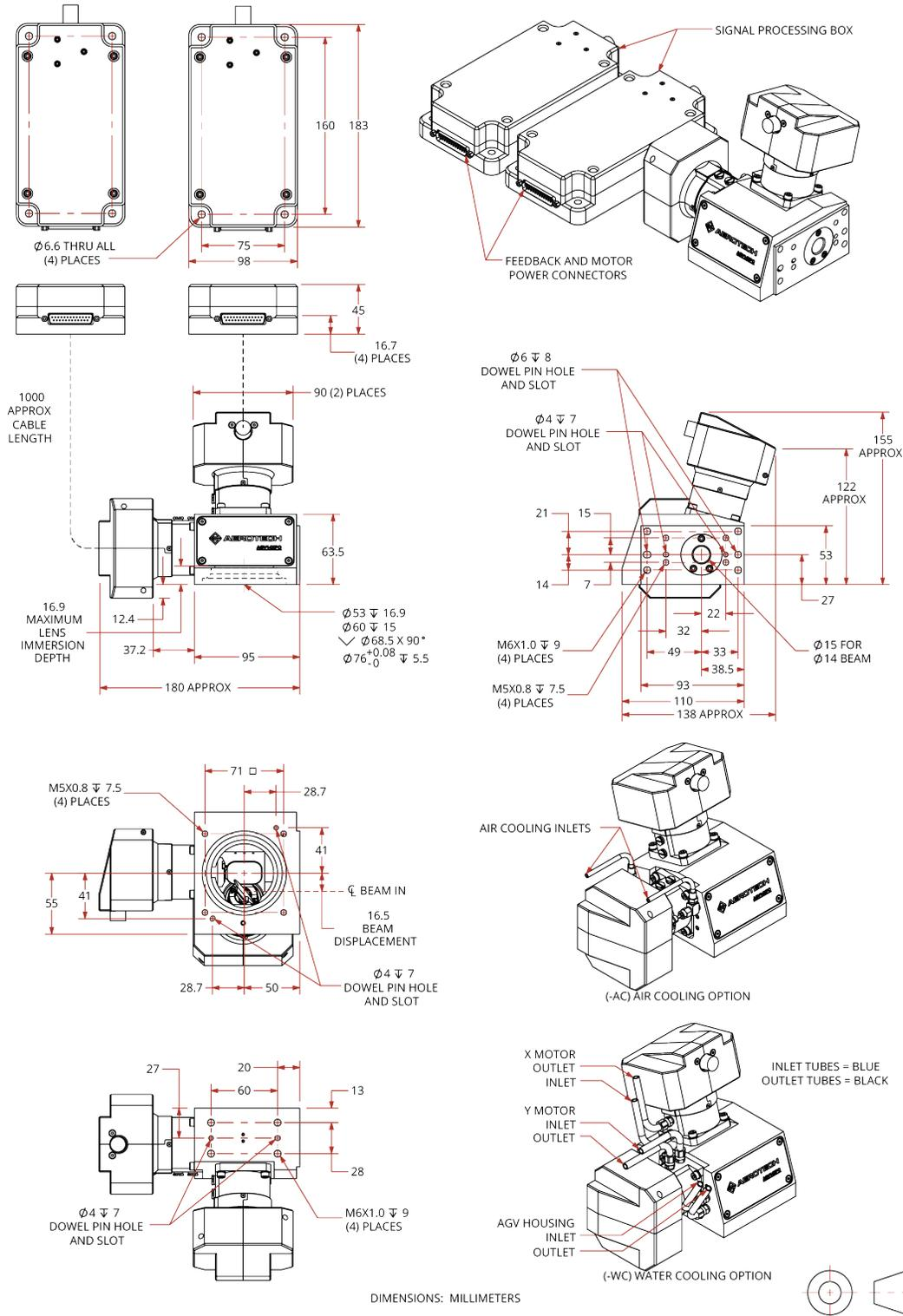
Figure 2-8: AGV14XPO-E2-BE2 Galvanometer Scanner Dimensions
