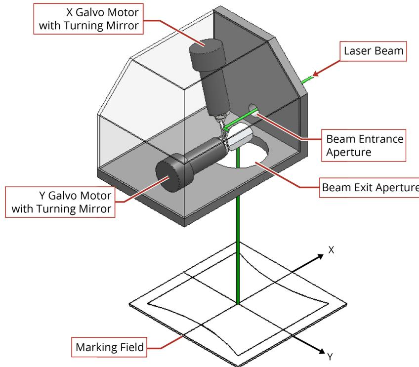
The AGV-HPO control connections are two 25-pin D-style connectors. The AGV-HPO is also available with right-side and left-side input apertures for “mirror image” machine builds or side-by-side scanner mounting with a single laser beam split to source both scanners.
