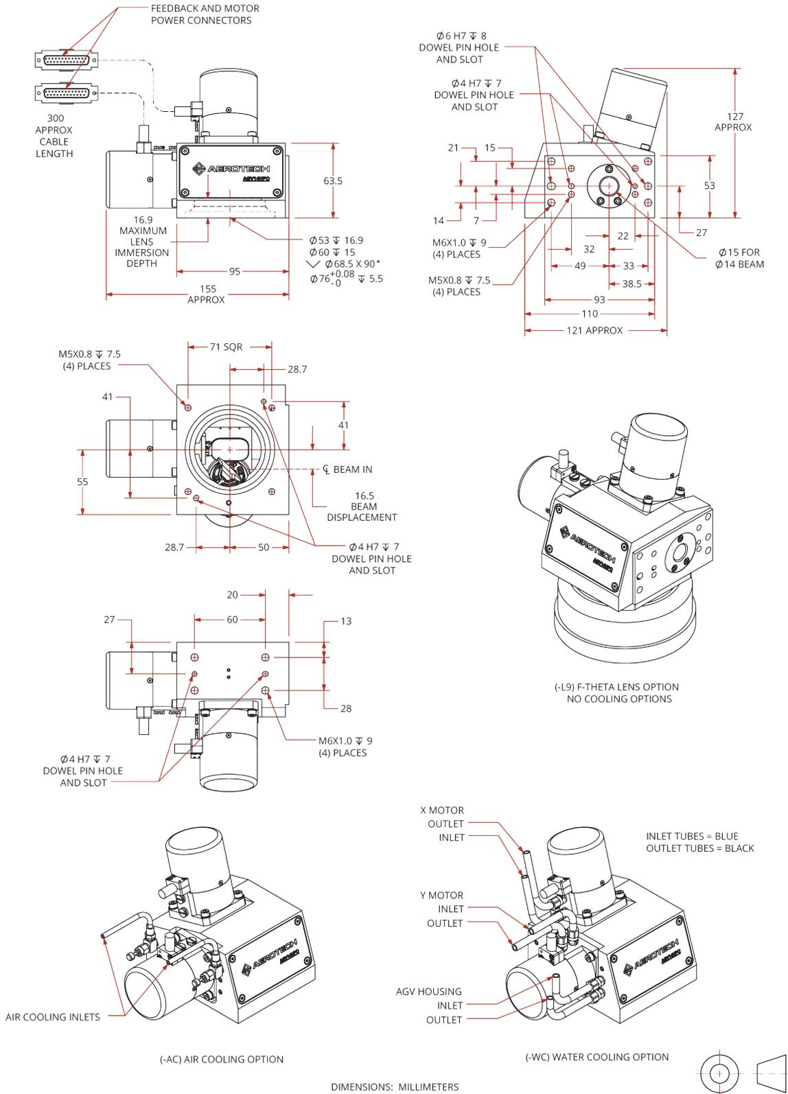
Figure 2-4: AGV14HPO-BE2 Galvanometer Scanner Dimensions
