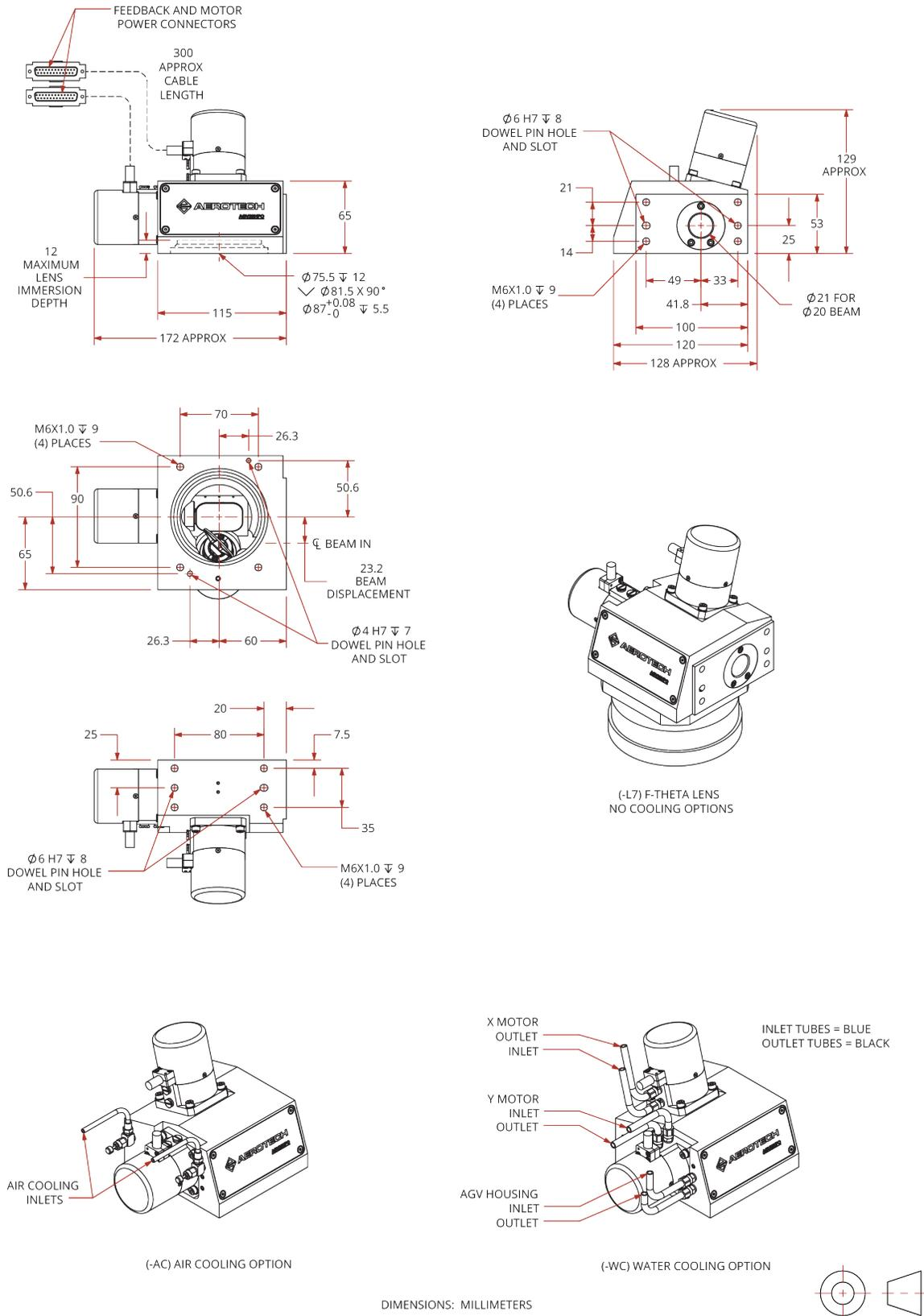
Figure 2-6: AGV20HPO-BE2 Galvanometer Scanner Dimensions
