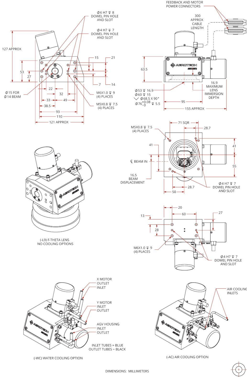
Figure 2-5: AGV20HPO-BE1 Galvanometer Scanner Dimensions
